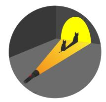
The farther an object is from a source of light, the smaller its shadow is.
